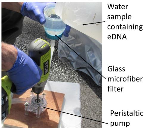
**Figure 1.** eDNA filtration being carried out in the field.
